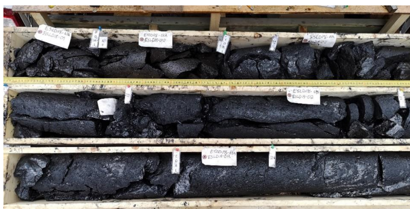
Figure 3. Large Diameter Core (LDC) samples from the first cored hole
