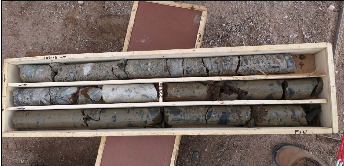
Figure 1: Diamond drill core from drillhole C-01-19, at ~273m showing brine bearing breccia-conglomerate host lithology
