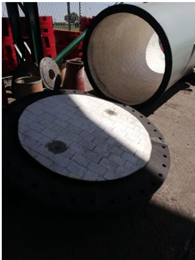
Mill shell and base ceramic lined
