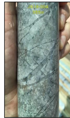
Molybdenite-quartz veins in dacite porphyry
