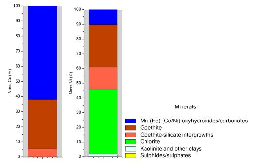
Figure 2: QEMSCAN elemental deportment for Cobalt and Nickel.
