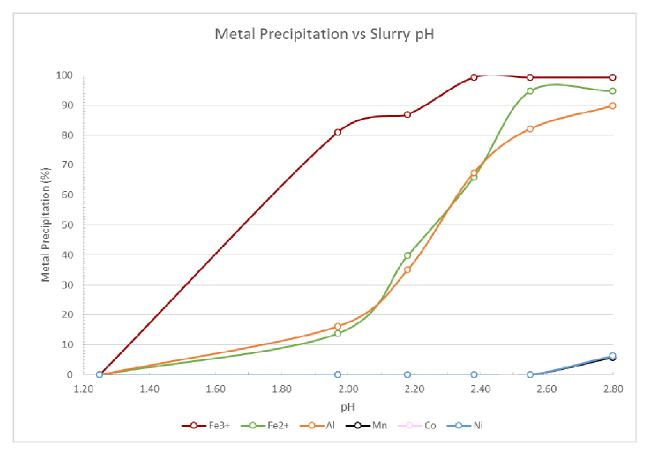
Figure 3: Neutralisation test HY7252 showing successful precipitation of iron an aluminium ahead of payable metal precipitation at pH 2.4-2.6.
