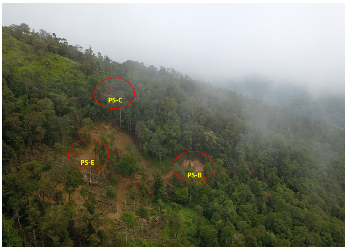
Figure 4: Aerial photograph of the Puncak Selatan prospect showing three prepared drill sites (the proposed Awak Mas open pit crest position corresponds to the ridge at top left corner).
