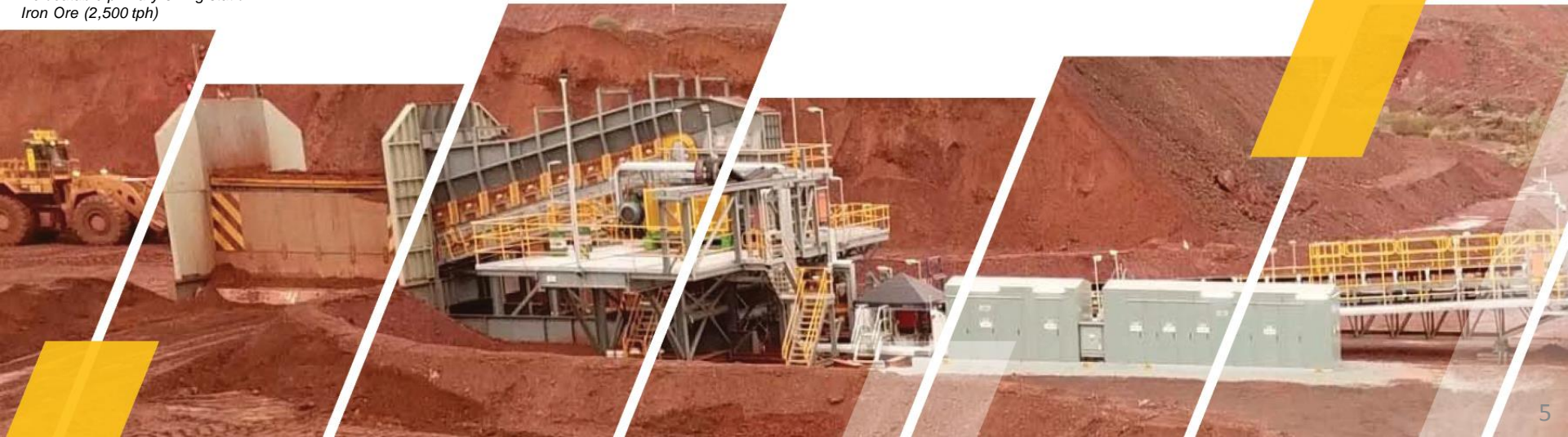
Relocatable primary sizing station Iron Ore (2,500 tph)
