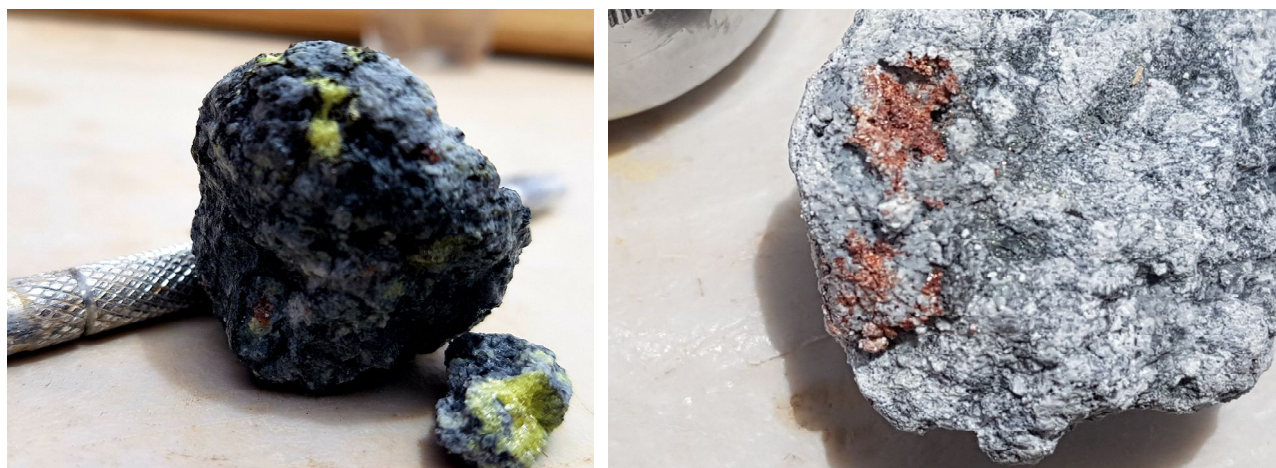
Figure 4 (a) Left: Native sulphur at 133m and (b) Right: Possible pyrrargyrite or pearceite, significant “ruby” silver minerals, in tuff breccia at 133-134m, both from hole 5100-2
