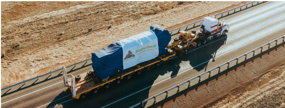
One of three Wartsila 34DF generators during the 3000km journey from Fremantle port to Tanami Gold Mine in the Northern Territory.
