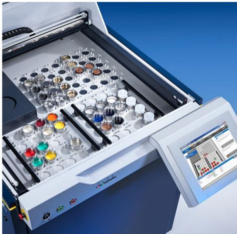
The glass disk is presented into an x-ray spectrometer for analysis
