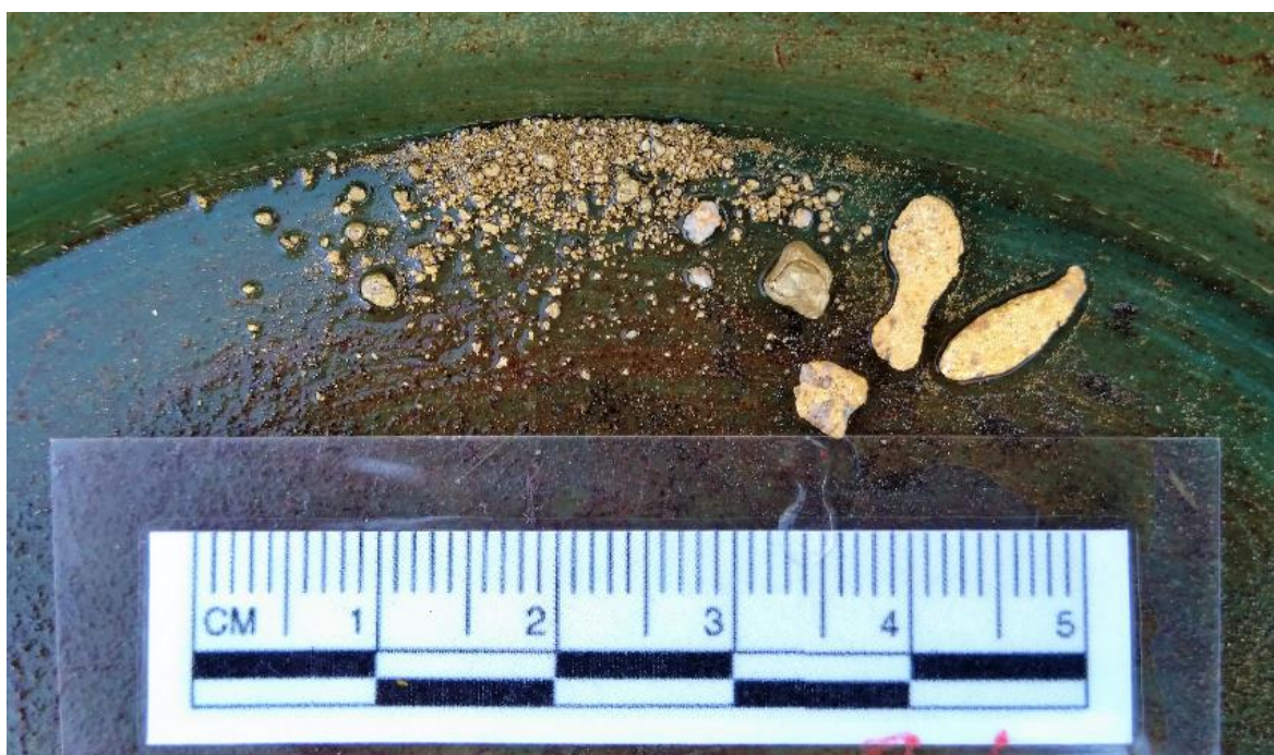
Figure 2 Loudens Trench LTR002 Sample LB250-021 - 1.083gms Au concentrate from 250kg sample
