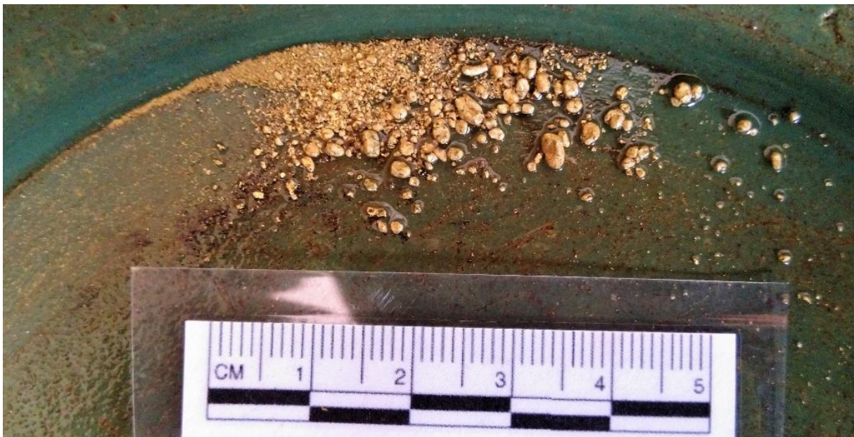
Figure 1 Loudens Trench LTR001 Sample LB250-007 - 1.502gms Au concentrate from 250kg sample
