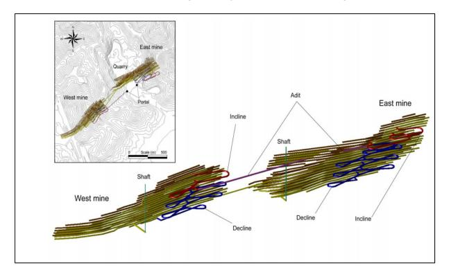
Figure 1 General layout of proposed underground access surrounding the quarry in Yogwang
