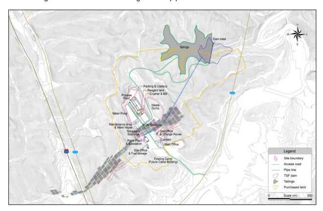
Figure 3 Surface infrastructure and mine layout
