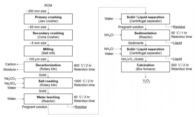
Figure 2 Proposed processing flowchart
