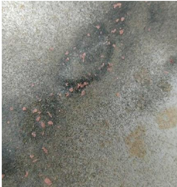
Figure 4: Native Copper Identified in the Stage Grind
