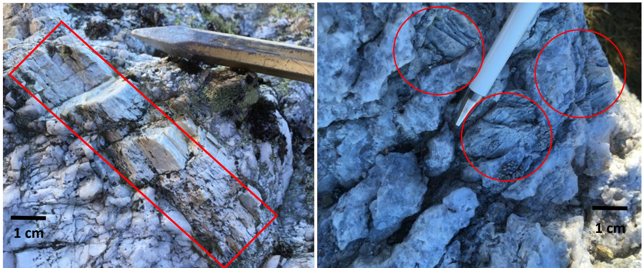
Figure 9 - Field samples with large spodumene crystals (up to 10 cm) embedded in a qtz-feldspar matrix. Figure left sample 75065 2.91% Li 2 O, Figure right sample 75091 2.06% Li 2 O.
