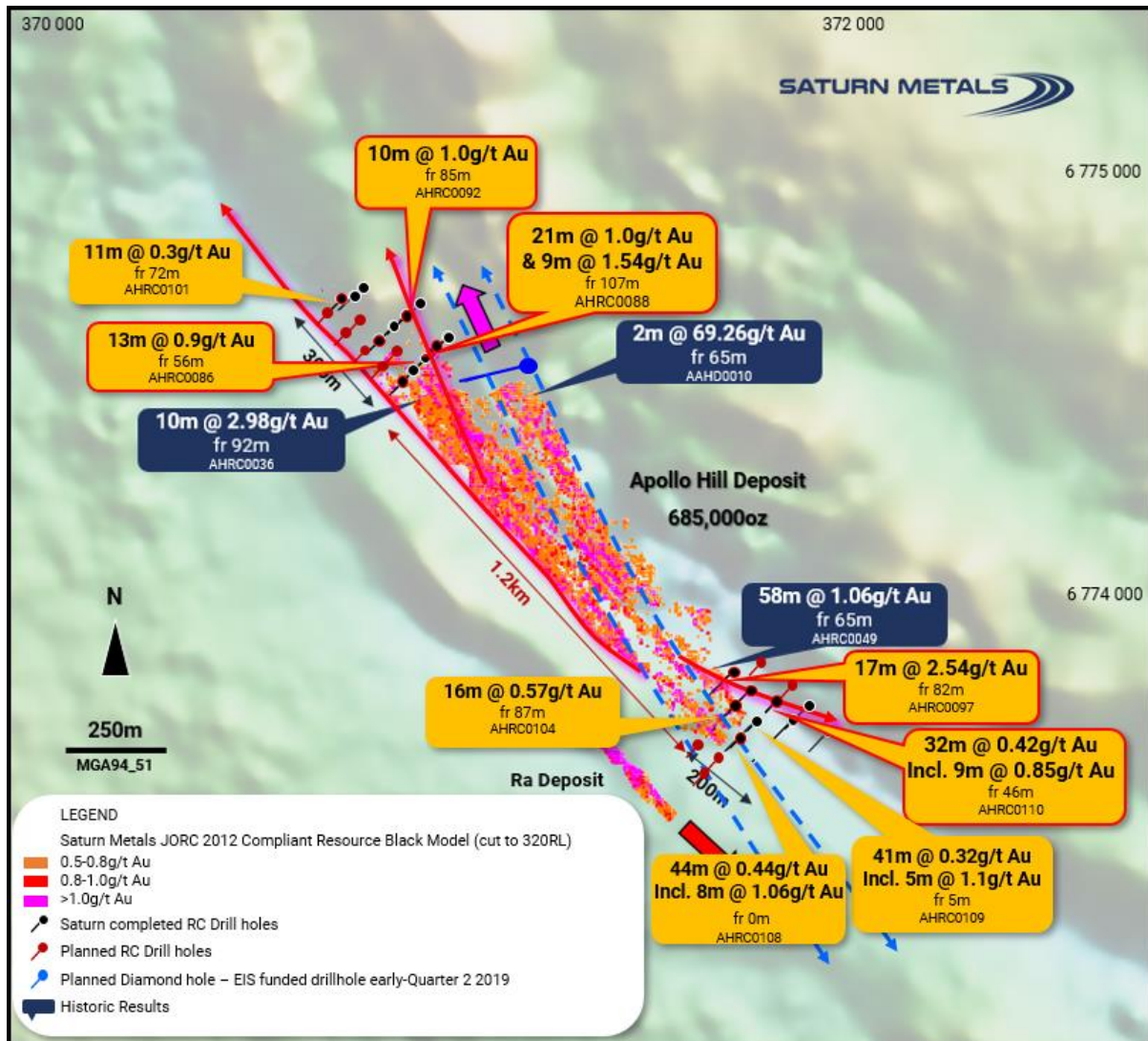
Figure 1 RC drill results relative to the published resource. Drilling results have expanded the 1.2km long mineralised system by an additional 500m strike length. Magnetic data collected in 2018 is providing a new targeting tool for future drilling. 2 Drilling results depicted originally reported in fuller context in Saturn Metals Limited ASX Announcements, Quarterly Reports and Prospectus - as published on the Company's website. Saturn Metals Limited confirms that it is not aware of any new information or data that materially affects the information on results noted.
