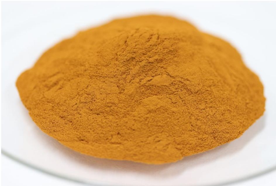
Figure 2: Photograph of High Purity 99.53% V_2O_5 Product from Gabanintha
