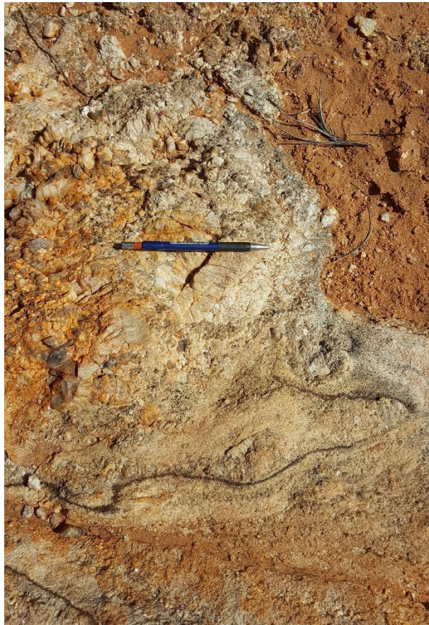
Plate 5. Outcropping pegmatite with both graphic and aplitic/saccharoidal textures (very fine crystalline groundmass) located at N7692068 E689145, GDA94, zone 50.
