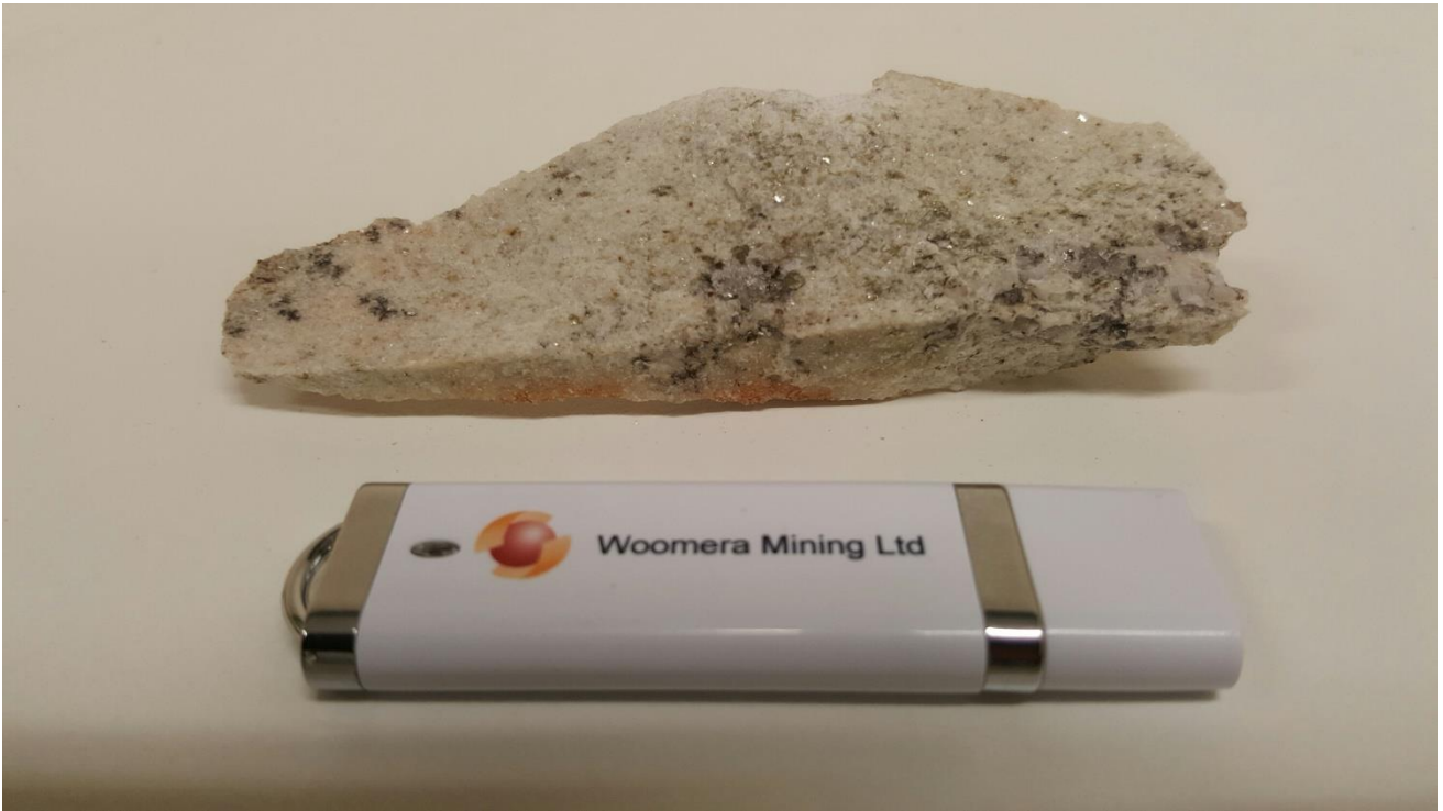
Plate 11. Rock chip sample MRR02-064 - saccharoidal quartz, feldspar, golden mica, beryl?, garnet and metallic aggregates in low angle vein within greisenised granite, located at E 689166 N 7692065 GDA94, zone 50.
