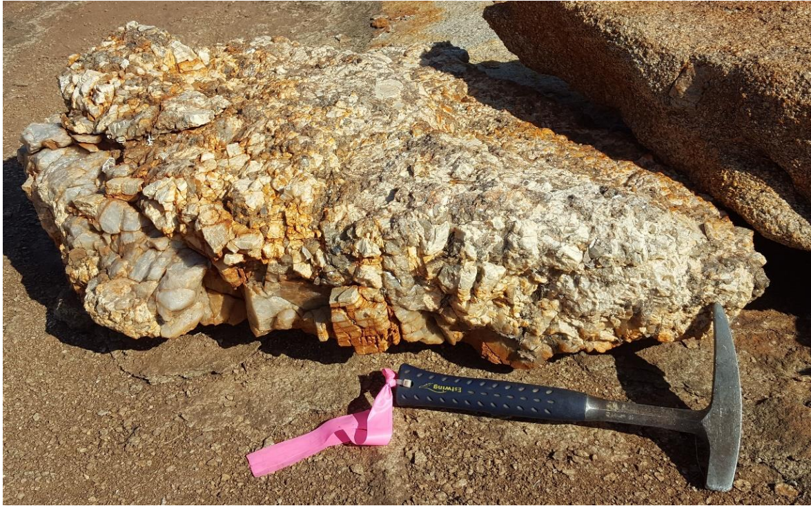
Plate 3. Coarse banded granitic pegmatite with well-developed feldspar and quartz crystals, near MRR02-016; located at N7687401 E690215 GDA94 Zone 50
