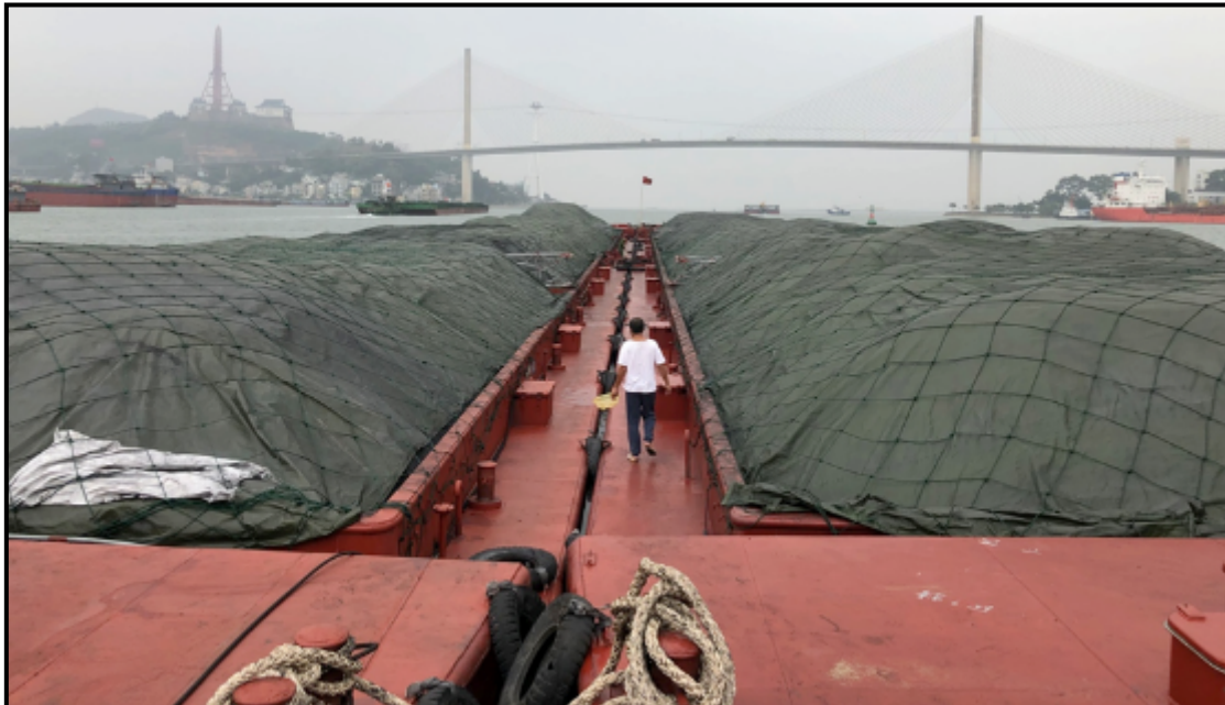
Four Shallow Draft Barges – 1,700 tonne Capacity each.
