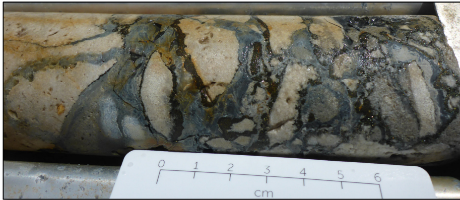
Figure 5 :Core from GSWA core library showing anomalous Zn in XRF up to 2% with pyrite within Barbwire Terrace tenements..
