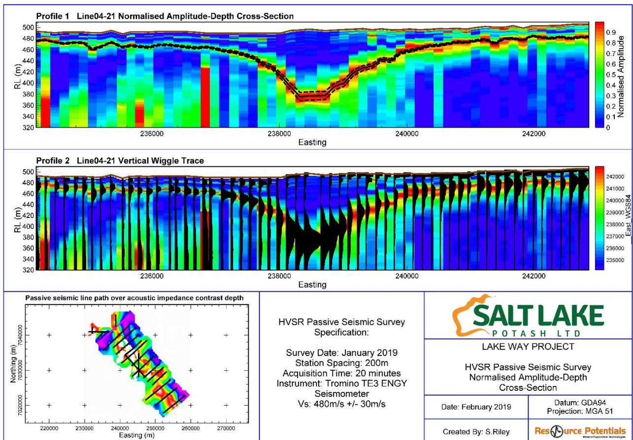
**FIGURE 13: INTERPRETED HVSr PASSIVE SURVEY DATA CROSS-SECTION FOR SURVEY LINE 04-21**
