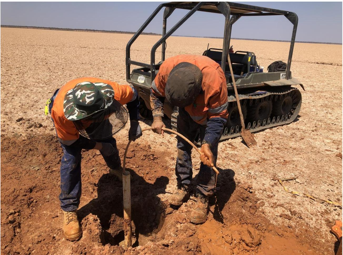
**FIGURE 6: SLUG TESTING A PIEZOMETER**
