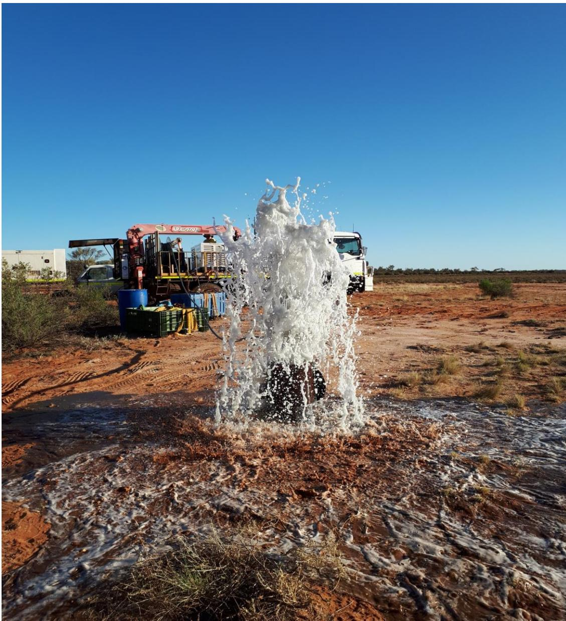
FIGURE 7: BORE TEST PUMPING AT LAKE WAY
