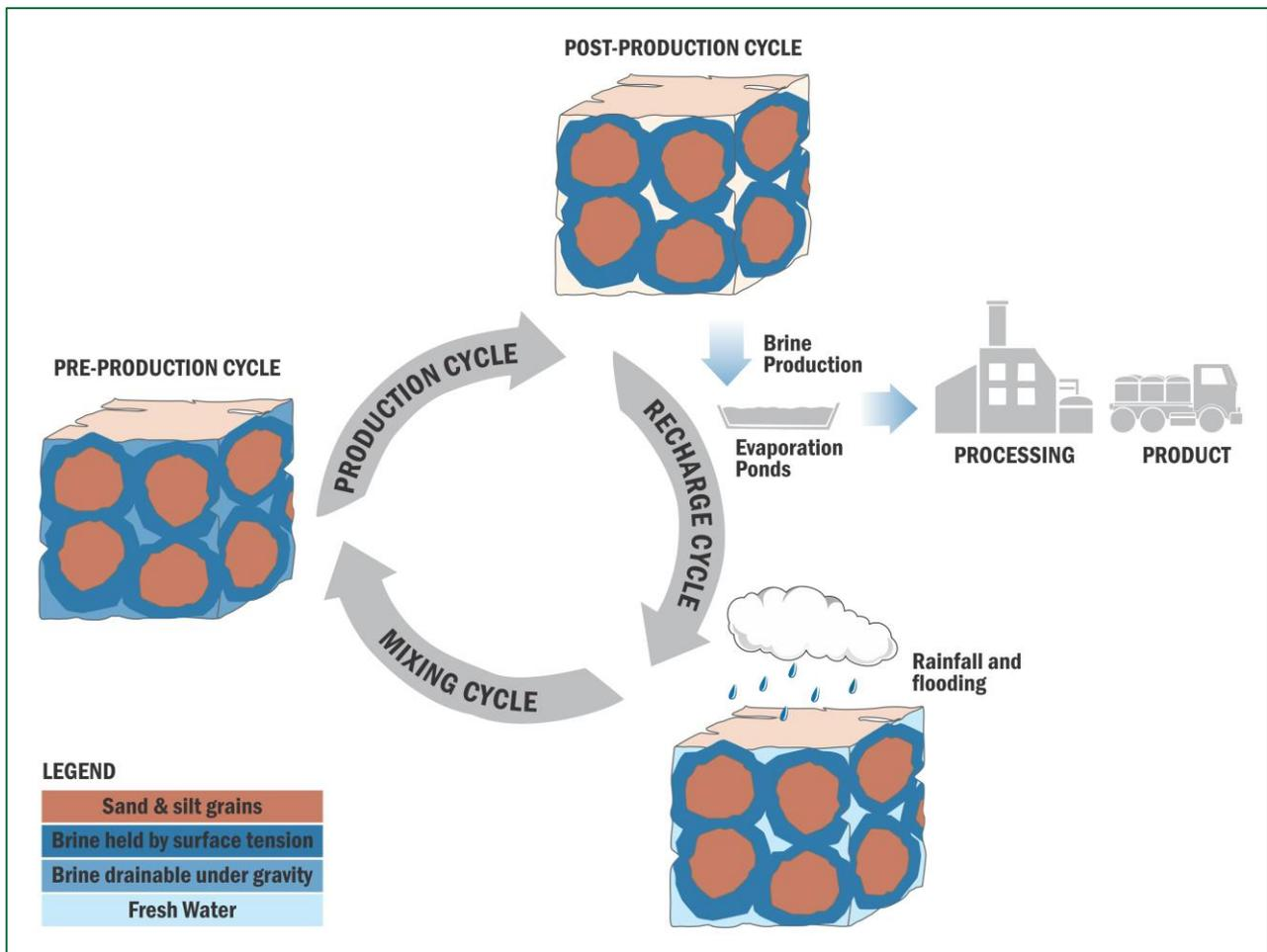
FIGURE 16: LAKE BED SEDIMENT SOP PRODUCTION CYCLE
