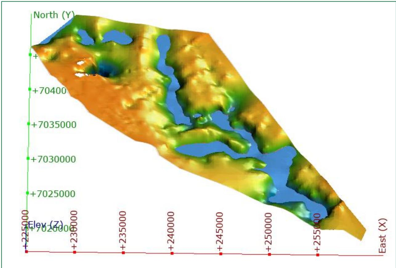
FIGURE 12: 3D VIEW OF BASEMENT MODEL WITH INTERPRETED BASAL SAND FILL (LOOKING NORTH)
