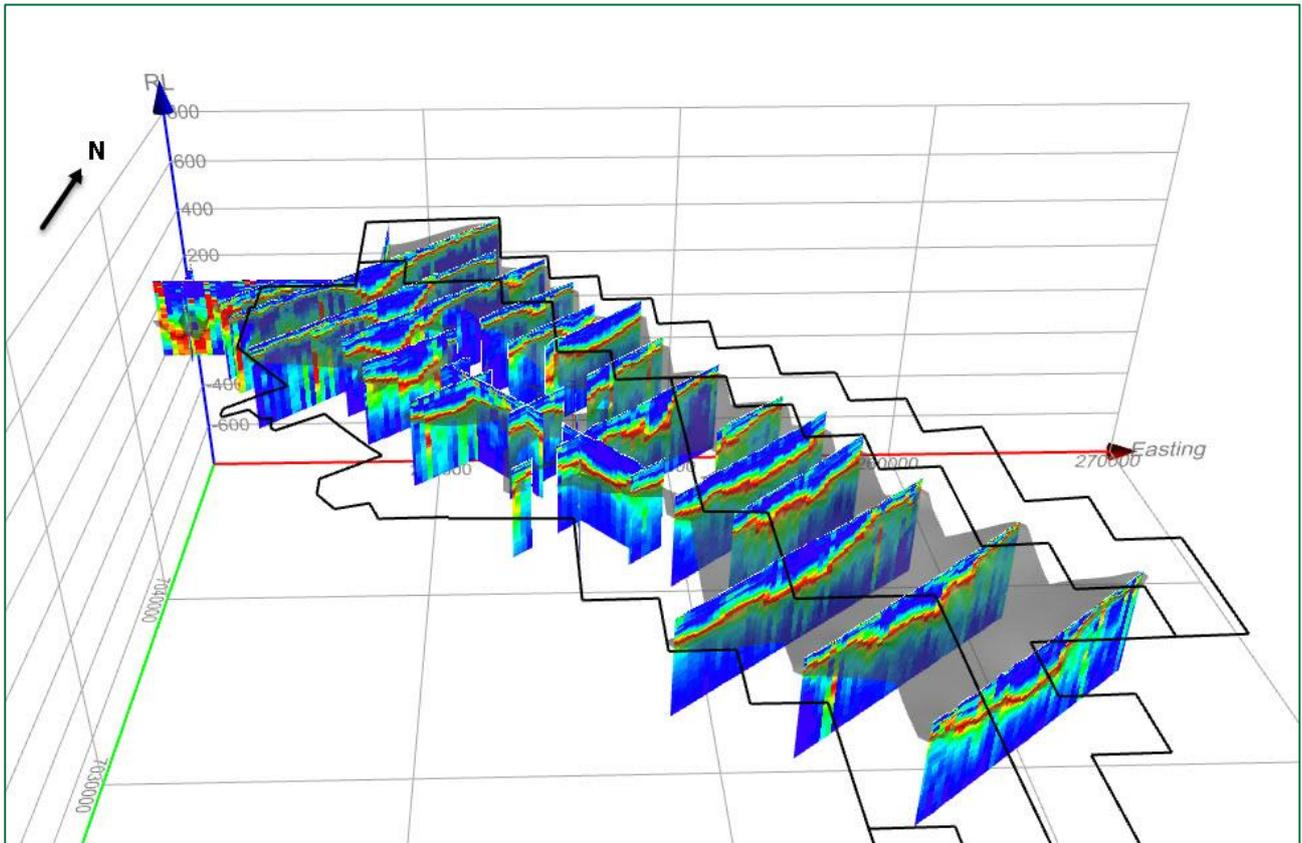
**FIGURE 10: 3D VIEW OF HVSR INTERPRETED CROSS-SECTIONS OVERLAIN WITH THE SALT LAKE POTASH TENEMENTS. LOOKING NORTH.**
