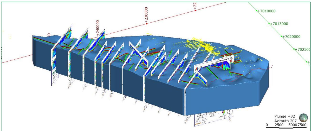
**FIGURE 11: 3D VIEW OF HVSR INTERPRETED CROSS-SECTIONS SHOWN WITH BASEMENT MODEL AND HISTORIC DRILLING DATA POINTS (YELLOW POINTS). LOOKING SOUTH WEST.**
