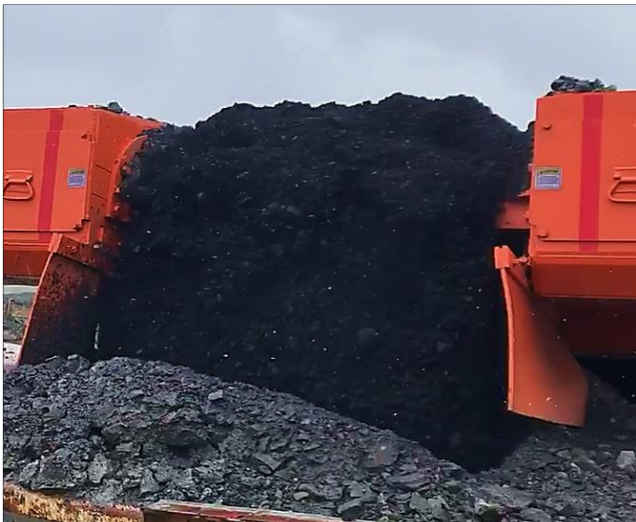
Figure 1: Surface feeder transferring coal from the Poplar Grove mine to the CHPP (image from video on Company website)
