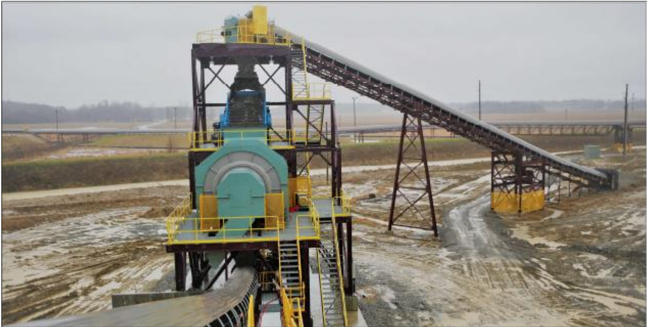
Figure 2: Raw coal reporting to the CHPP ROM screen and rotary breaker
