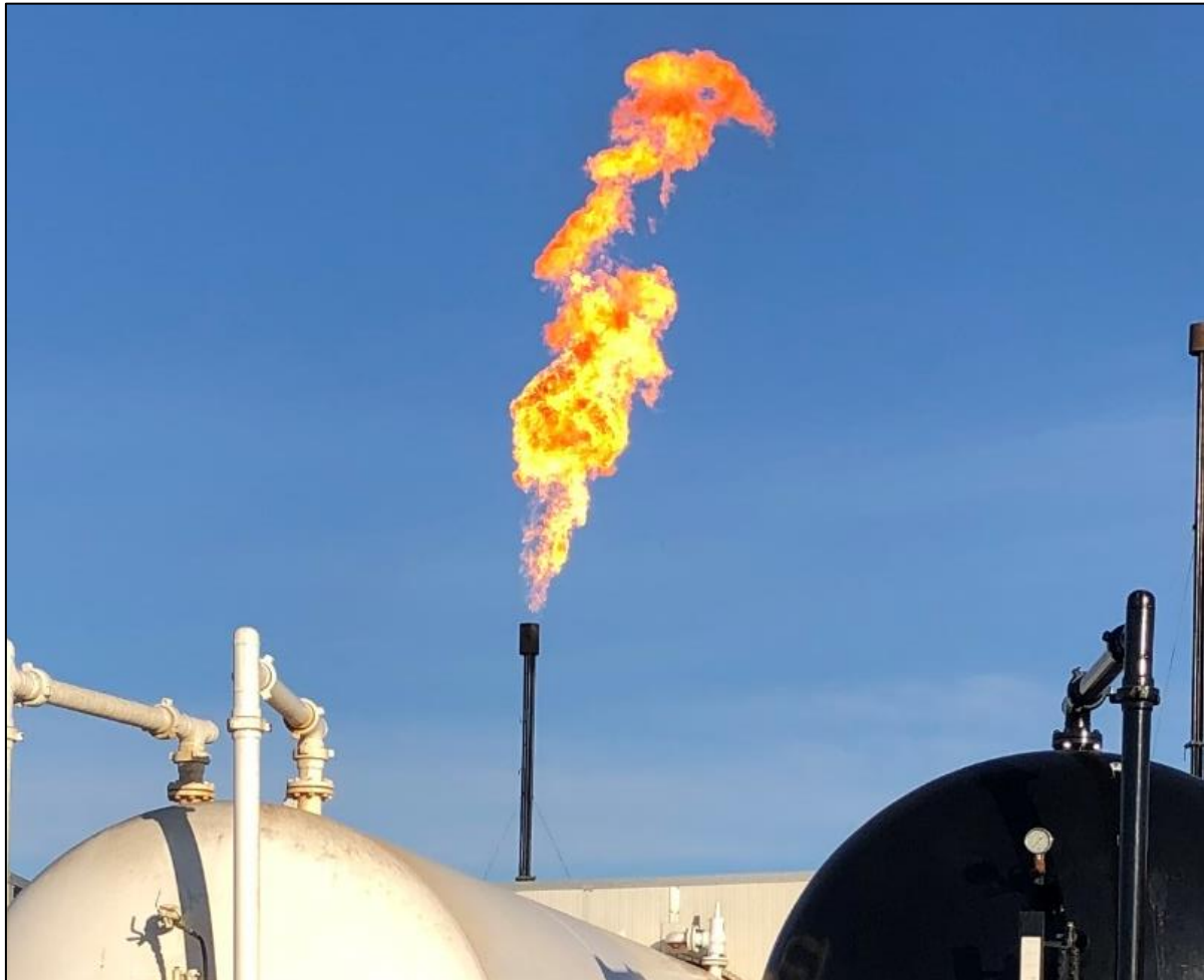
Figure One – Gas being flared during initial testing operations of the Calima-2 well.
