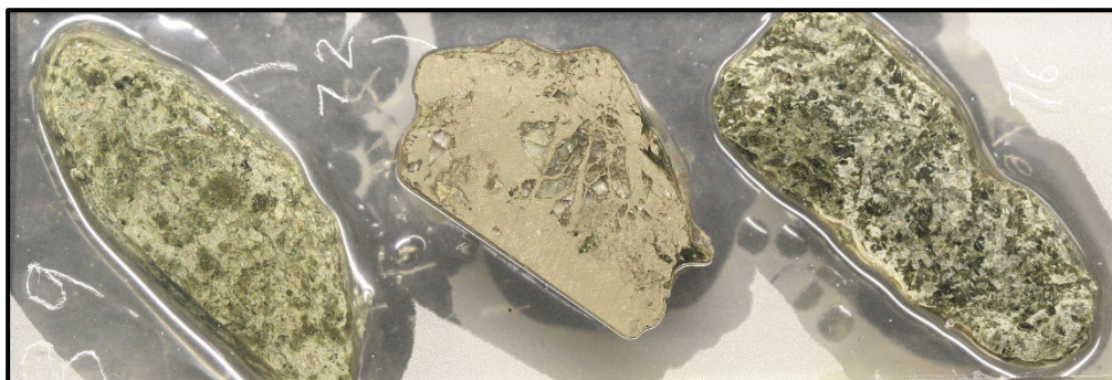
Figure 1 – Sulphide chip in centre (slide height = 26mm) with mafic host rock on either side (LAAC039 from 71 metres)
