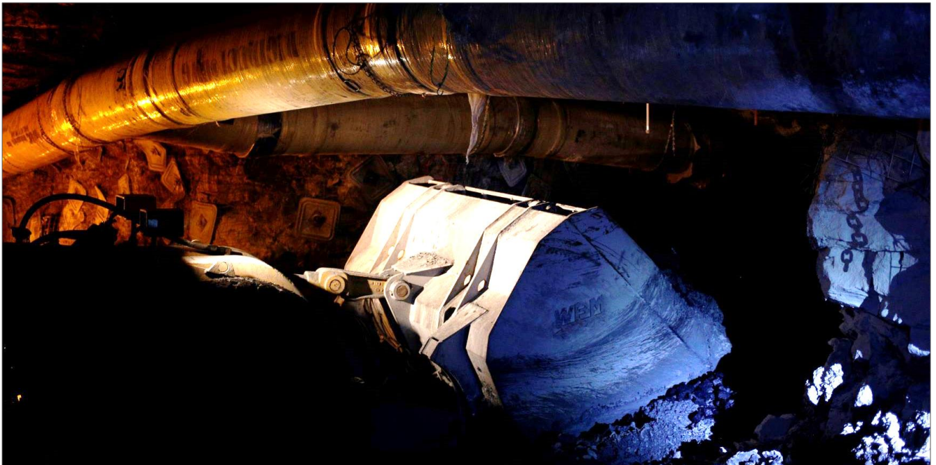
Image 2: Paringa loader mucking RoM material from the mine face
