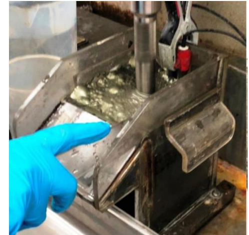
Cleaner flotation test and resultant filtered base metal concentrate
