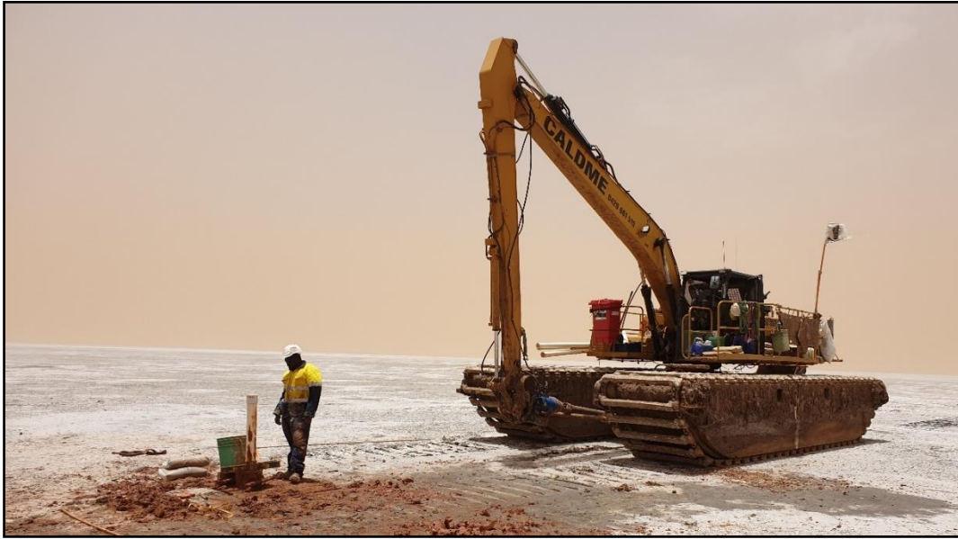
Auger-equipped AM315 Amphibious Excavator and a completed bore
