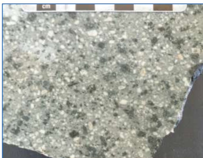
Figure 7.6 Dacite Hand Specimen *
