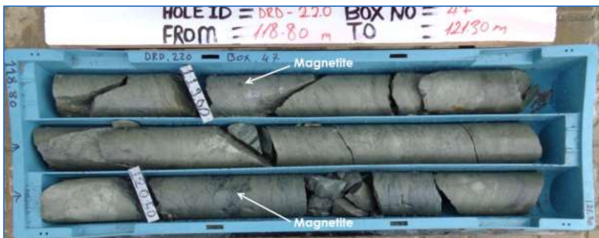
Figure 7.20 Magnetite Aligned with Schistosity in Core
