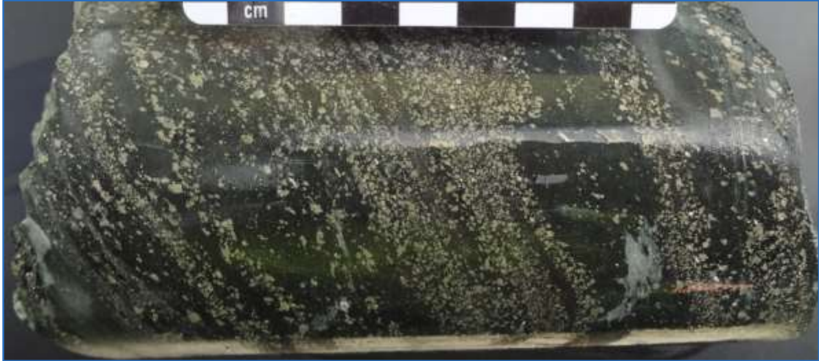
Figure 7.12 Chlorite–Sericite Schist Altered to Tr–Sulp Core Photograph
