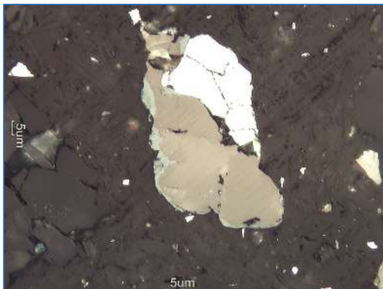
Figure 9.9 Pyrite Attached to Grey Sphalerite Rimmed with Blue Covellite and Chalcocite and Galena
