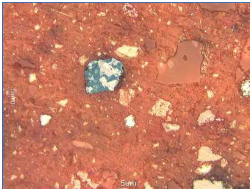
Figure from Polimetal, 2018. (* Covellite surrounded by iron oxide and silicates: Reflected light, 500x).
