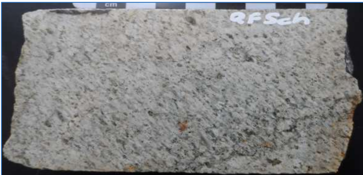
Figure 7.9 Quartz–Feldspar Schist Core Photograph
