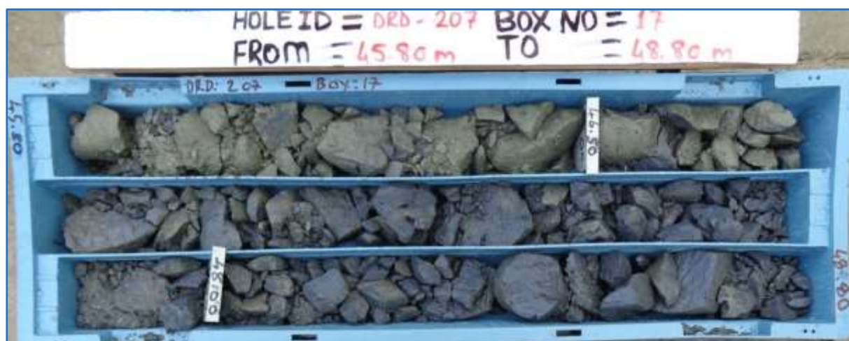
Figure 7.21 Enriched Mineralisation in Drill Core (Blue Colour)
