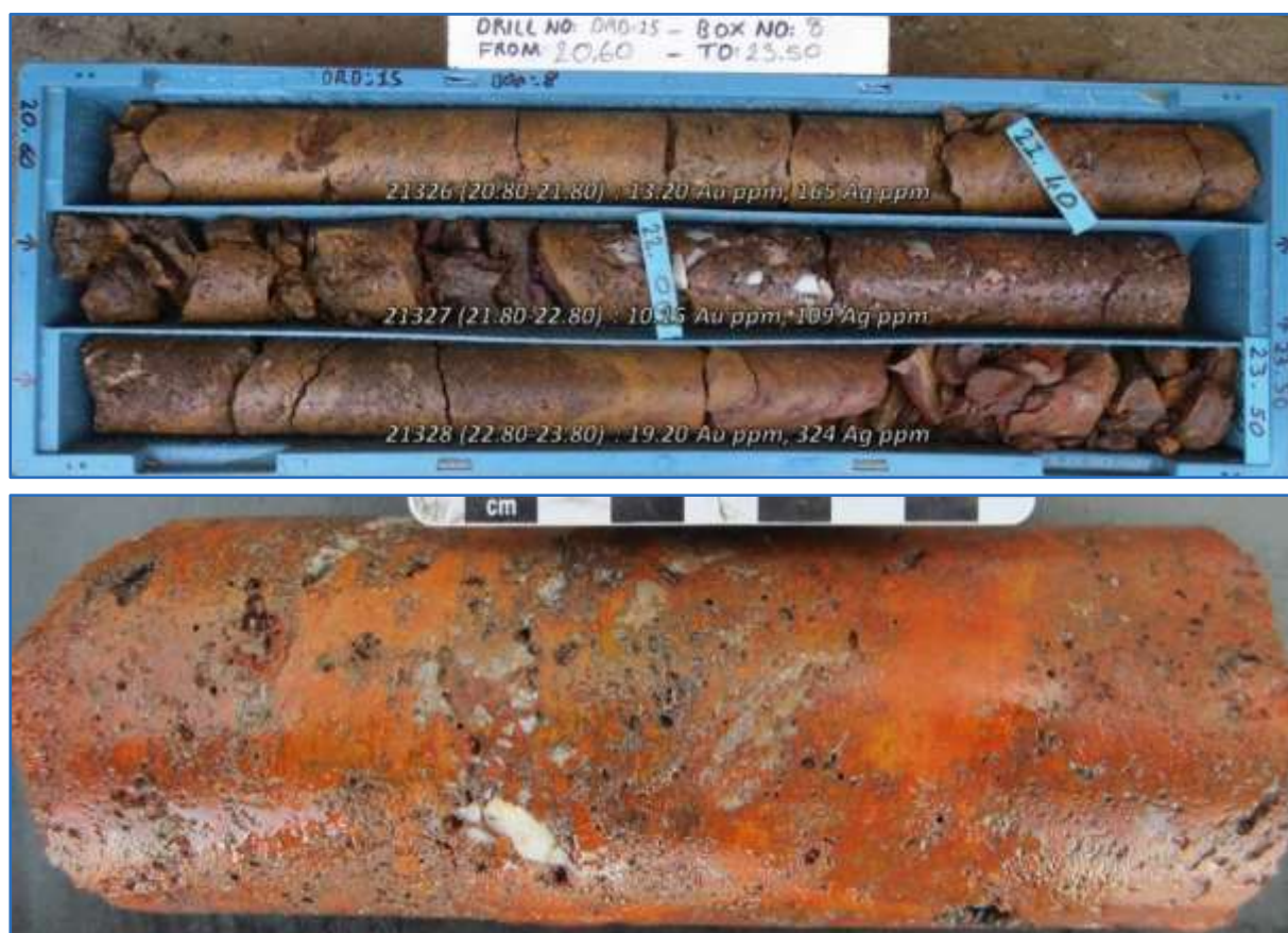
Figure 7.18 High-Grade Gossan Mineralisation Drill Core
