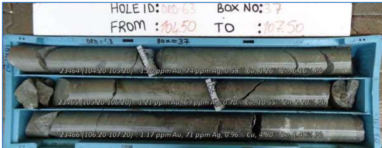
Figure 7.19 Massive Pyrite Drill Core
