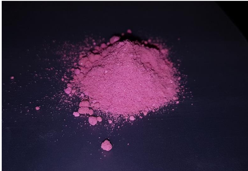
Image 1. Cobalt sulfate produced using First Cobalt Refinery flowsheet
