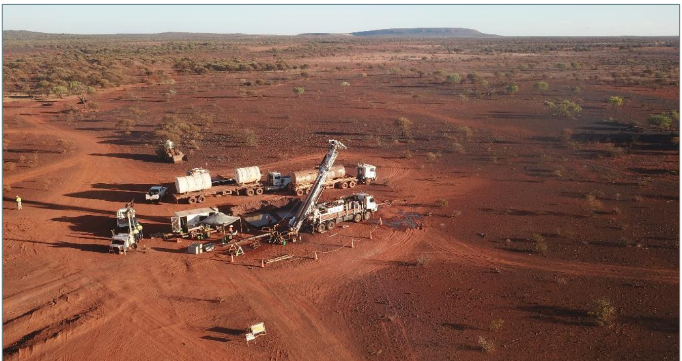
Plate 1 - Diamond drill rig on site at the Australian Vanadium Project
