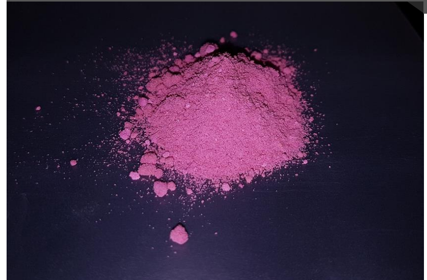
Cobalt Sulfate Produced Using First Cobalt Refinery Flowsheet
