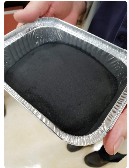
Magnetite concentrate after the first step in the TIVAN® process
