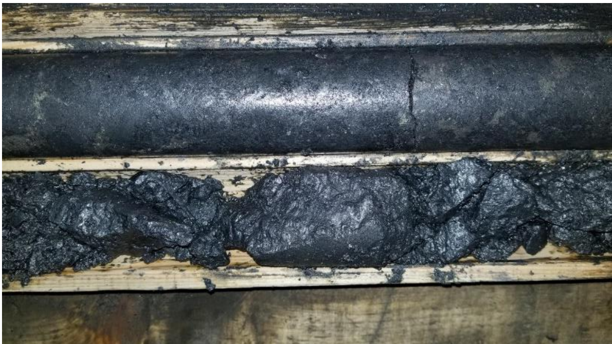
Figure 3 (right): Close-up of the main graphitic zone encountered in DDH LR19-05, illustrating a solid drill core graphite intersection ( top of core box ) and a fractured / broken graphite intersection ( bottom of core box ), Lac Rainy Graphite Project
