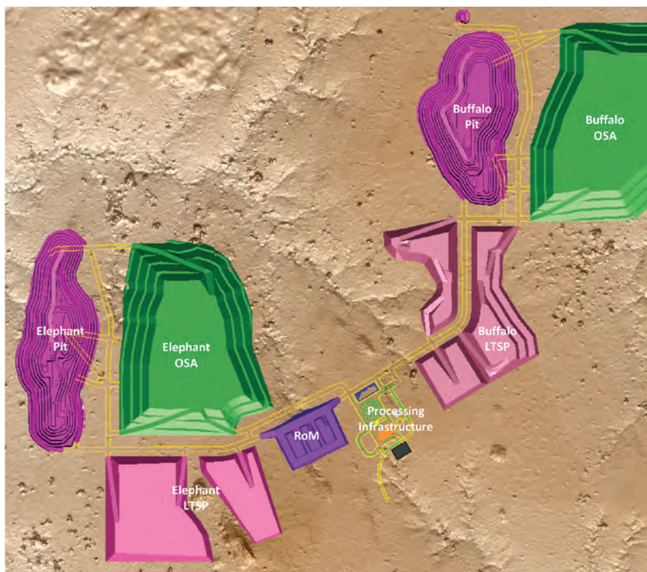
Figure 2. Montepuez Graphite Project: Mine & Processing Site Layout.
