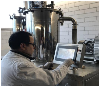
Figure 12: Spheronising unit at the German facility and Laser particle sizer chart showing the narrow particle size distribution of spherical graphite.
