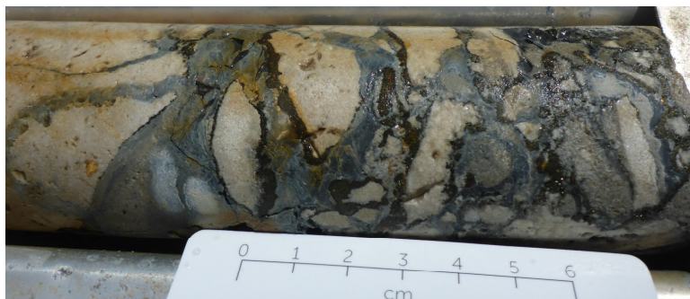
Figure 6: Close-up of WRD01 at 495.3m showing carbonate breccia hosted mineralisation with 2% Zn spot XRF with marcasite.
