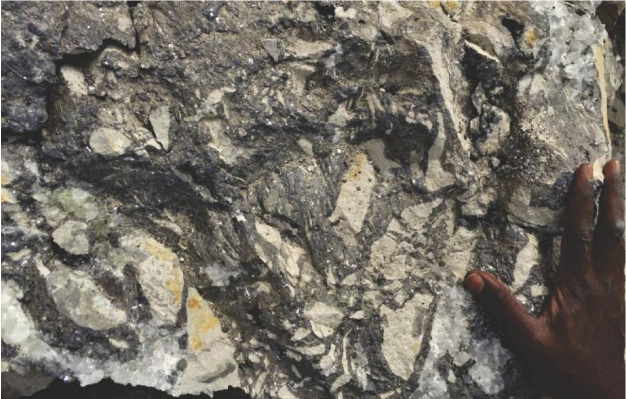
Figure 3. High-grade sphalerite breccia ore at the 275mRL in the Macy Pit (approximately 25m below surface level). Sphalerite (ZnS) is the dark matrix material to the paler sandstone fragments.
