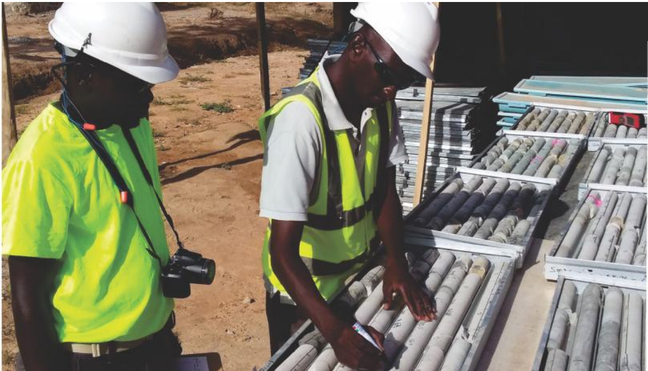
Figure 5 shows Nigerian geologists, Tijjani Machina and Nazifi Abdullahi conducting geophysical test work on the Macy core to determine the petro-physical characteristics ahead of the Company's ground Induced Polarisation (IP) survey.
