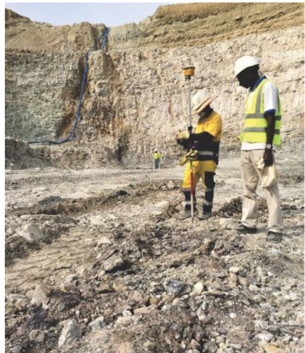
Figure 6. View of the north wall of the Macy Pit from the 280mRL, looking along the strike of the mineralisation to the north. Notice the near-vertical Macy Fault in the pit wall and the darker blocks of high-grade sphalerite on the floor in the foreground.
