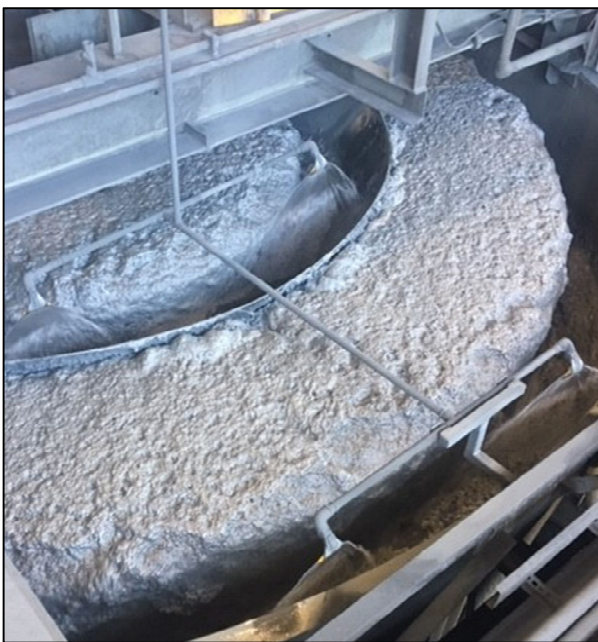
Figures 3 & 4: Launder sprays for the cleaner circuit (left) now operational (end of March 2019) and installation of pipe racks as part of the refurbishment and upgrade of launder spray and reagent dosing systems (right)
