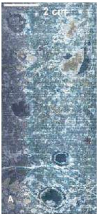
Plate 1: Black Swan orebody, drill hole BSD064. Coarse grained hopper-textured serpentinised olivine orthocumulate, showing subspherical segregation vesicles (black) partially filled by subspherical sulphide blebs 1
