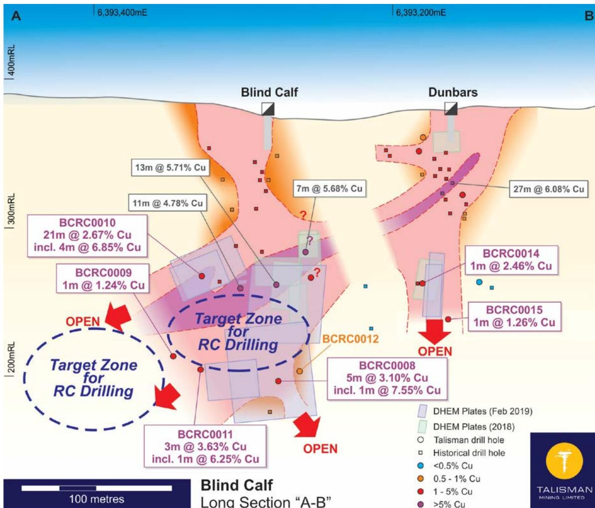
Figure 1: Blind Calf-Dunbar long section showing previously reported DHEM anomalies<sup>1</sup> and previously reported Talisman and historic drill intersections<sup>2</sup>.
