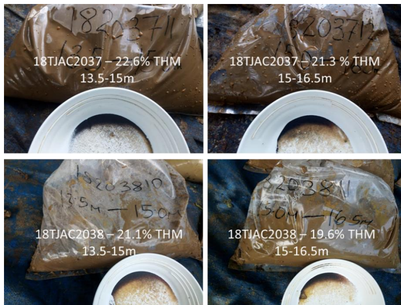
Figure 8 Panned samples from holes 18TJAC2037 and 18TJAC2038 within the Tajiri trap site. Photos show the bagged samples as drilled and panned from the field with the laboratory derived THM analysis superimposed over the image.
