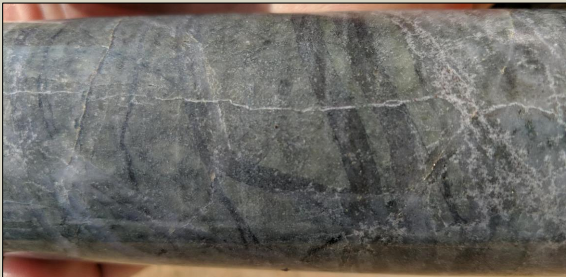
Photo 5. Porphyry M veins in a dacite at ~1,230m in SMD045.
