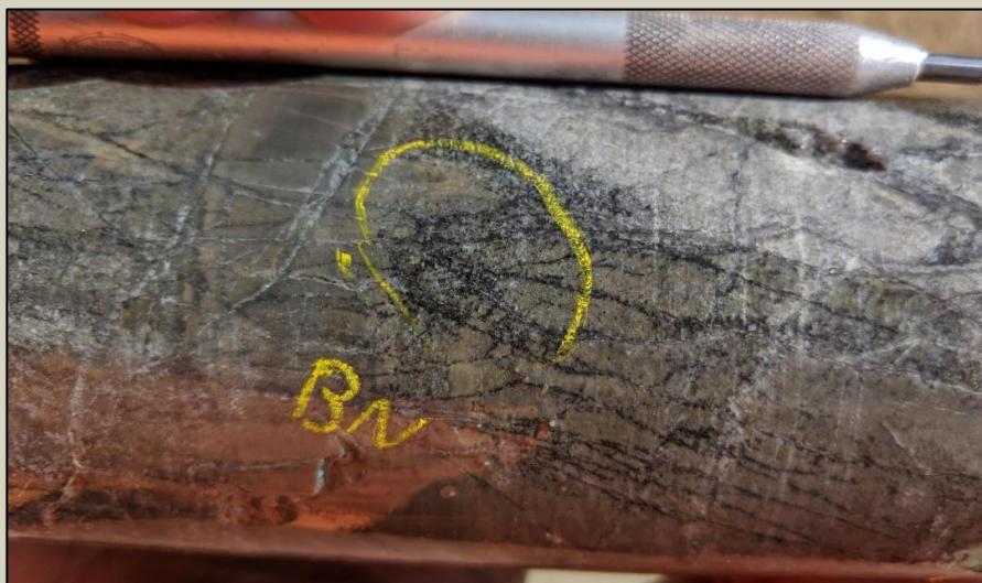
Photo 8. Fine bornite and chalcopyrite in 1mm wide quartz veins at 467.6m in SMD046.
