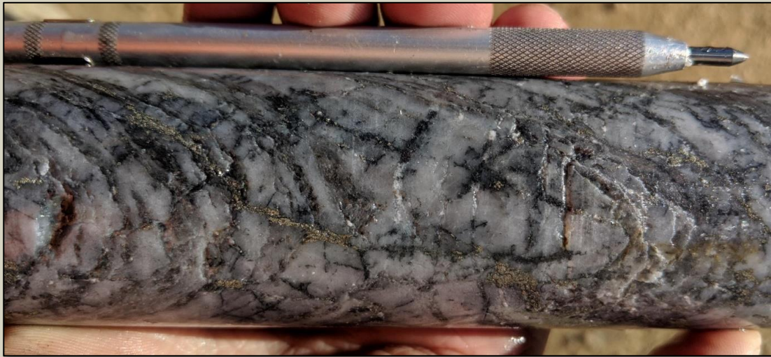
Photo 4. Laminated quartz vein, possibly once with magnetite, cut by pyrite and later finely intergrown bornite-chalcocite (dark patches) at 1086.5m in SMD045.
