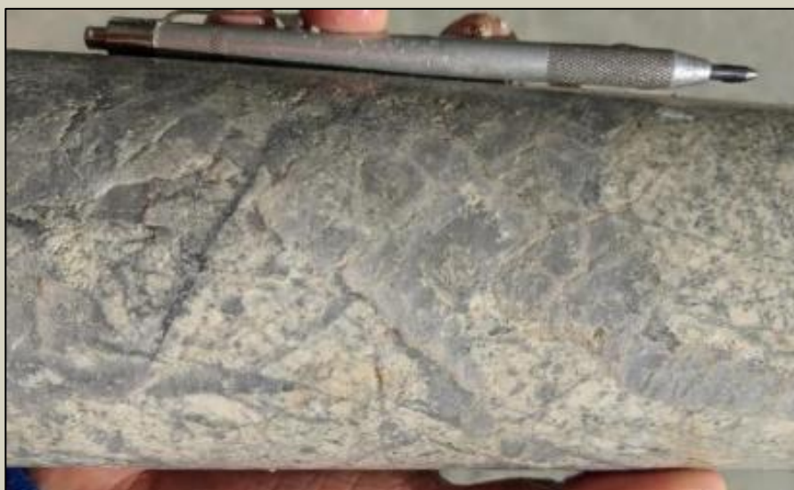
Photo 7. Well-developed quartz vein stockwork at 199.5m in SMD046.
