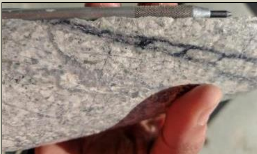
Photo 6. Quartz molybdenite veining in argillic altered quartz diorite porphyry at 188m in SMD046.
