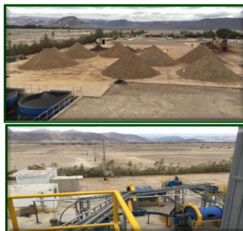
Figures 1 to 3: Vista Gold Plant – Leach Tanks for gold recovery (left), Crushed ore stockpiles ready for grinding and processing (upper right), and ball mill grinding circuit and conveyor feed to leach tanks (lower right)
