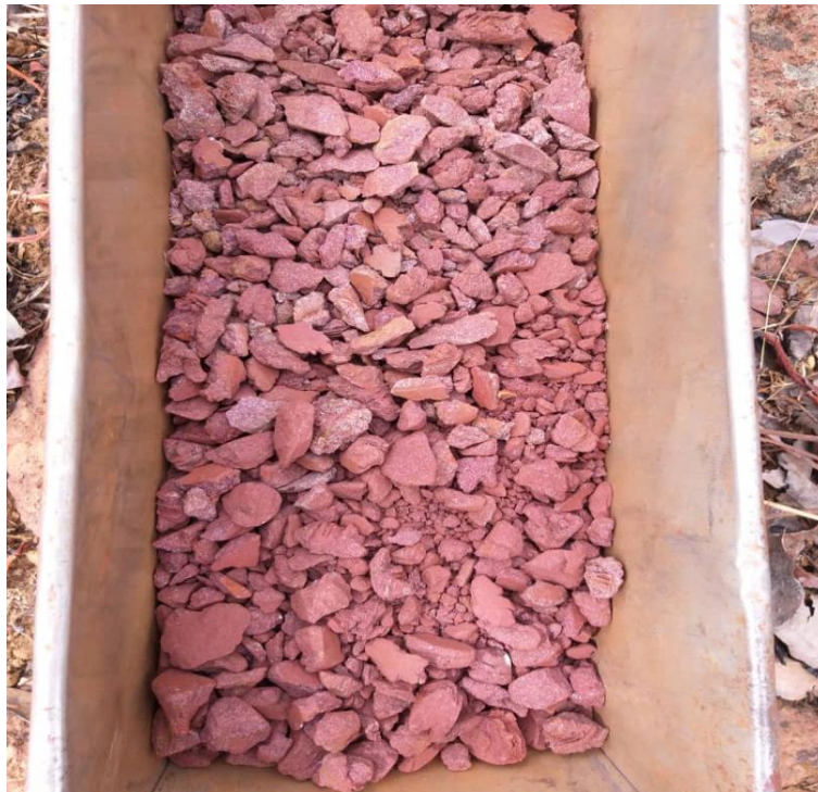
Figure 3: Recent drill core from Minim Martap showing visible gibbsitic bauxite.
