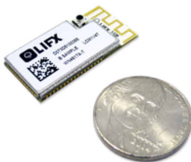
Figure 4 - The tiny LIFX Control Module (LCM), the “brains” behind each LIFX light.
