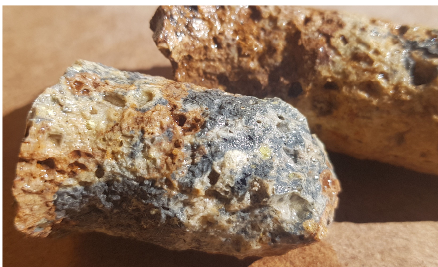
Figure 1: Core sample of fresh and oxidised vuggy silica from depth of 33 meters Hole 5300-8. Interval grades 3.5 g/t gold, within wider interval of 24m at 5.04 g/t gold 28.3 g/t silver from 20m. Note the presence of yellow native sulphur.
