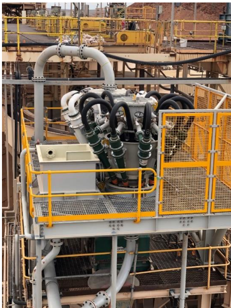
Figure 3. De-sliming and water recovery cyclone clusters on existing tailings screen
