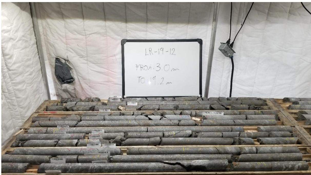
Figure 1: Semi-massive graphite flakes mineralisation intersected in DDH LR19-12 which intersected a zone of graphite mineralisation over a width of 26.6m graphite mineralisation (apparent thickness) at a depth from 3.0m to 29.6m. The image depicts the zone over a shorter interval from 3.0m to 19.2m, contained within this wider zone of semi-massive graphite flakes mineralisation
