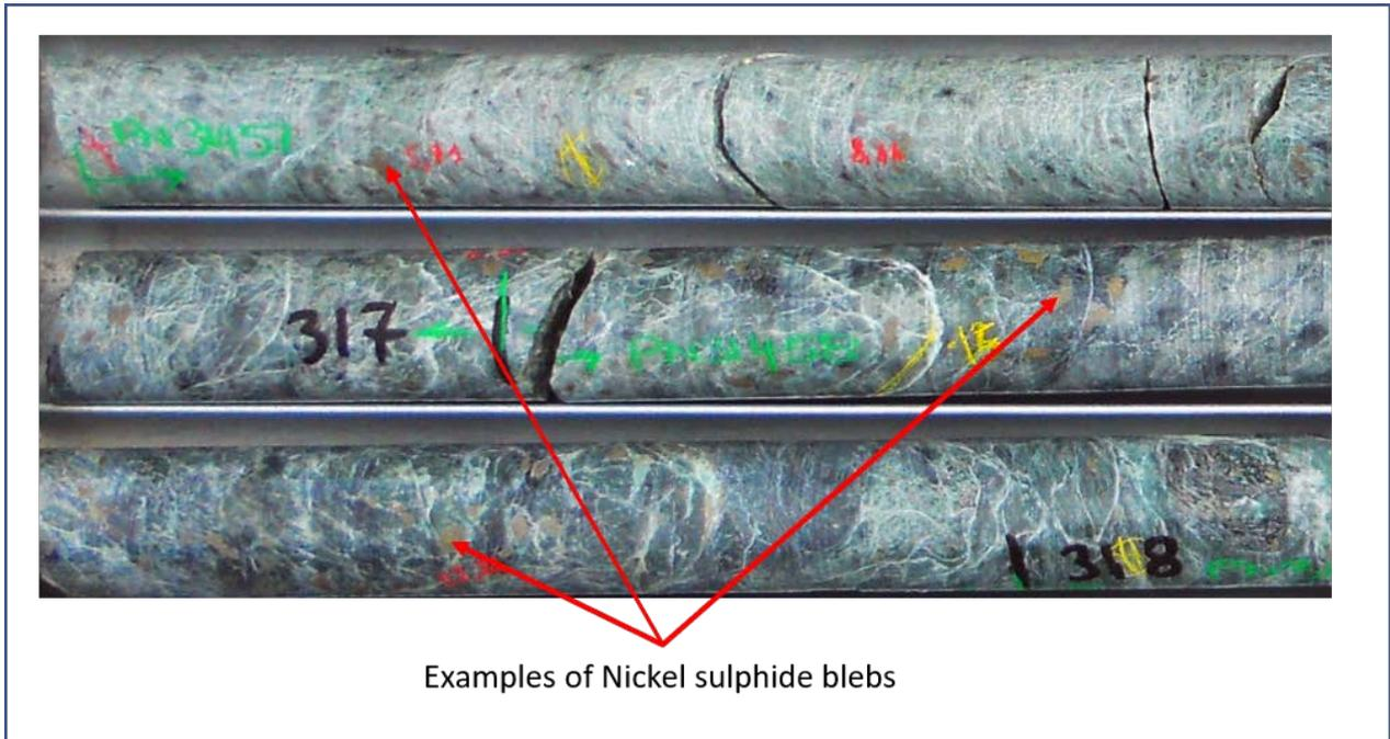
Figure 2- Core from PBSD001A showing blebby sulphide mineralisation (sulphide blebs up to 20mm in width) within competent ultramafic
