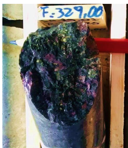
Photo 2: Traces of mixed primary sulphides (chalcopyrite and bornite)* on fracture planes in altered andesite at 329m in Hole 1
