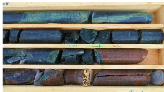
Photo 2: Traces of mixed primary sulphides (chalcopyrite and bornite)* on fracture planes in altered andesite at 329m in Hole 1
