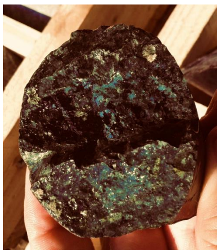
Photo 1: Traces of mixed pyrite and copper oxides* on fracture planes in altered andesite in Hole 1
