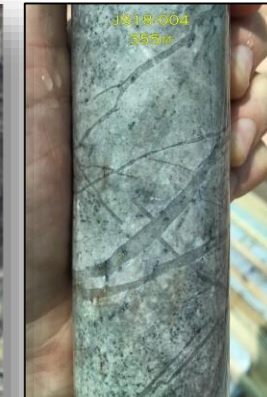
Molybdenite-quartz veins in dacite porphyry
